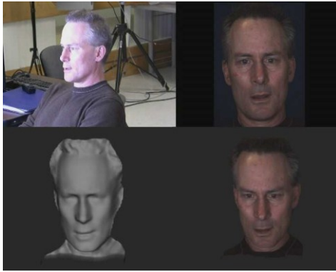
Figure 1: Upper-left: general view from a regular camera; Upper-right: 2D video; Lower-left: 3D dynamic geometric model; Lower-right: 3D dynamic geometric model with mapped texture.
