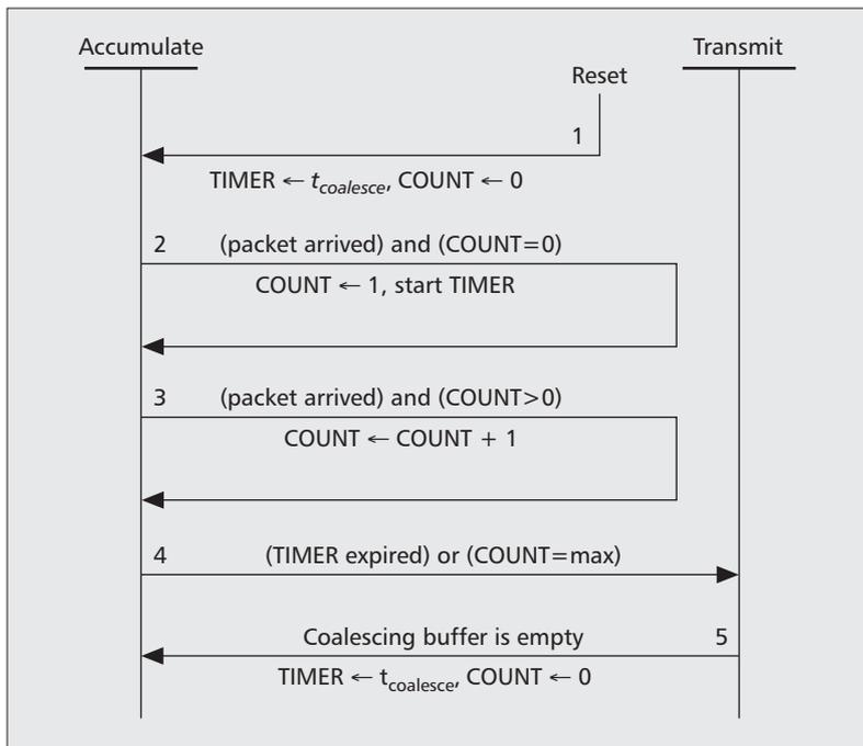
Figure 2. Finite state machine for packet coalescing.
