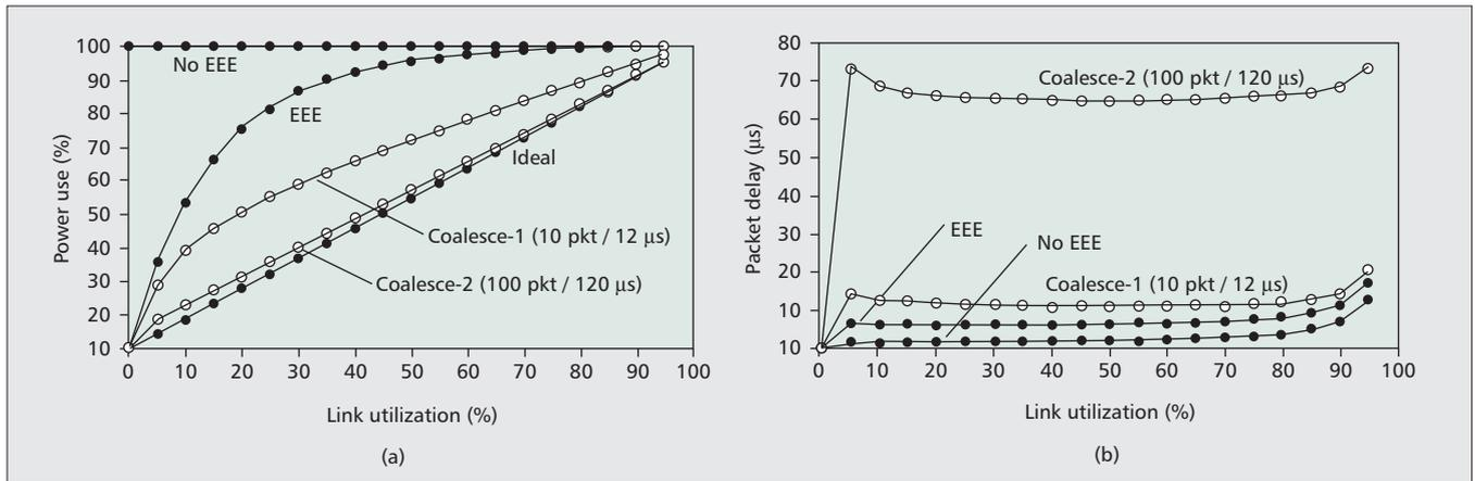
Figure 3. a) Energy use vs. link utilization; b) packet delay versus link utilization.
